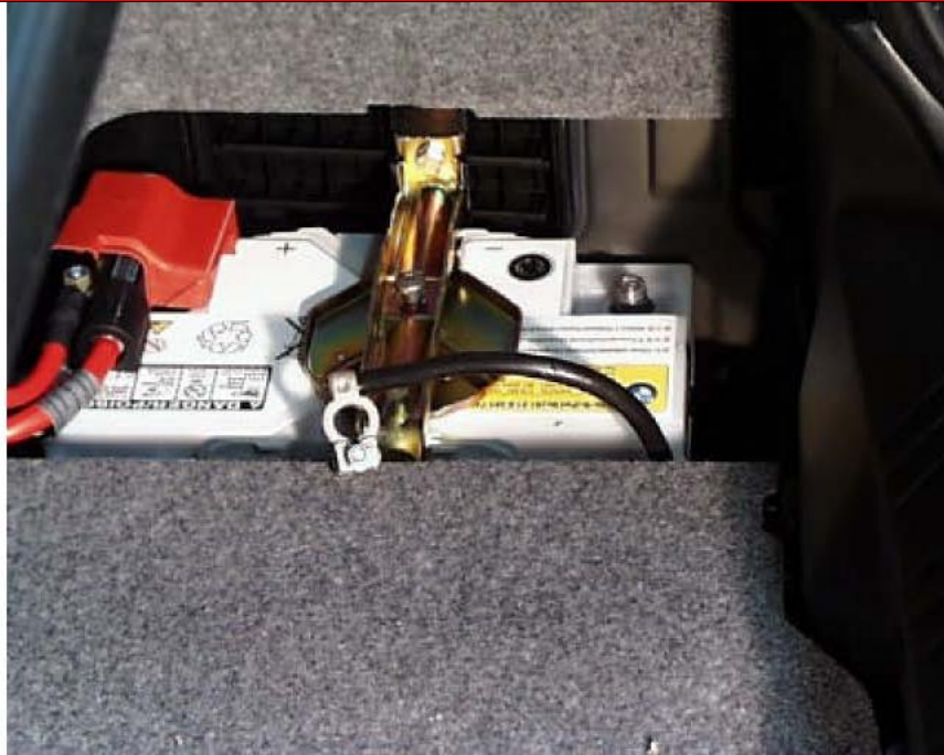
Figure 1 Disconnect the Negative terminal on the battery.
