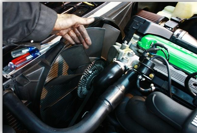
Figure 2: Spin Fan off by hand
