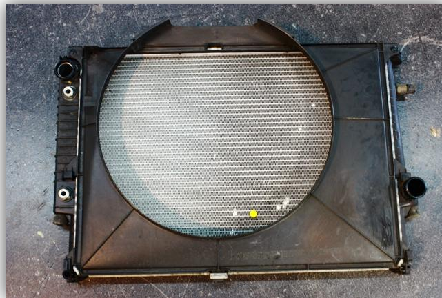
Figure 11: E34 Radiator removed
