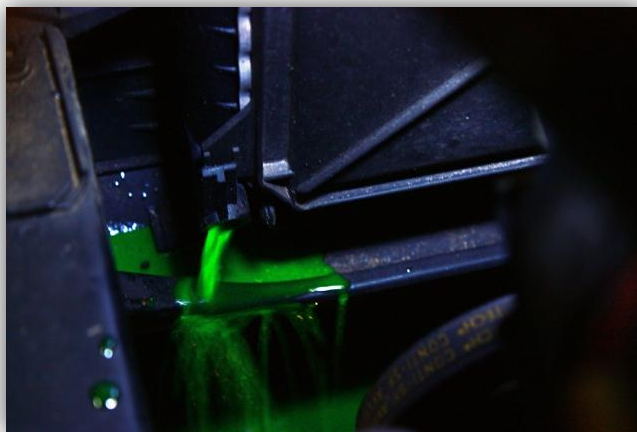
Figure 7: Coolant draining from radiator
