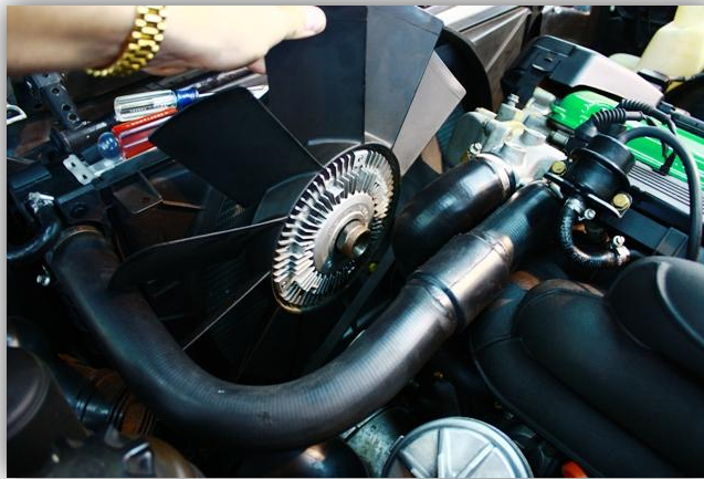
Figure 3: Remove Clutch Fan Carefully
