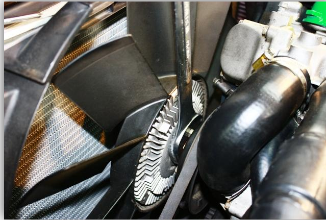
Figure 1: Crack Threads loose
